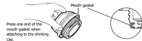
※The bottle will leak if the gaskets are not properly installed.
